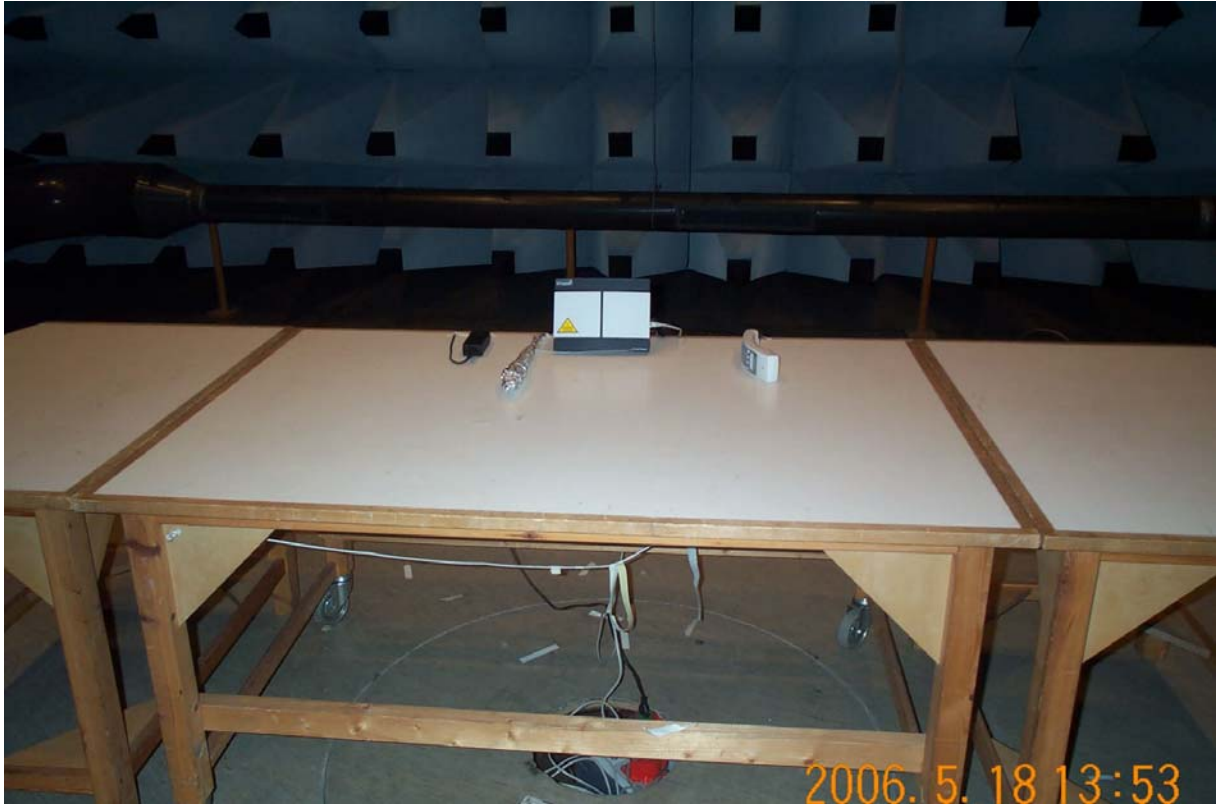
Photo A2.5 Radiated unwanted emission, BGAN MES radio.
