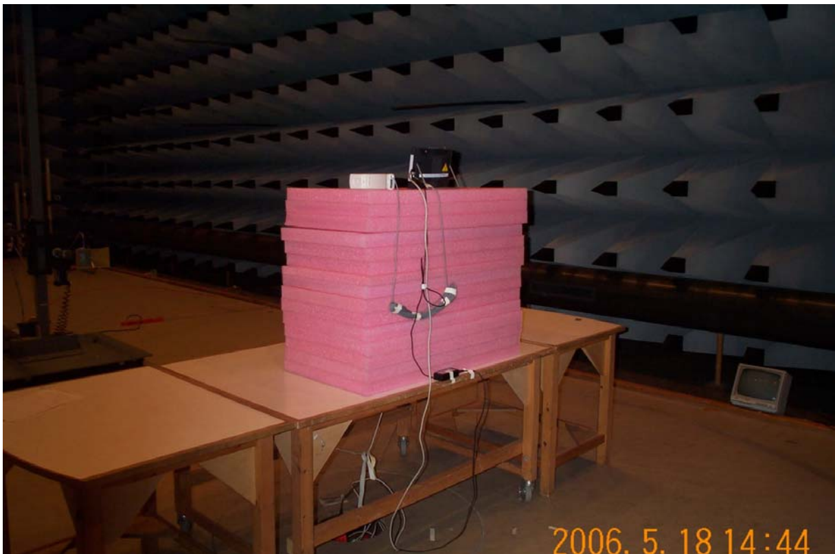
Photo A2.2 Equivalent isotropic radiated power (EIRP), Bluetooth module.
