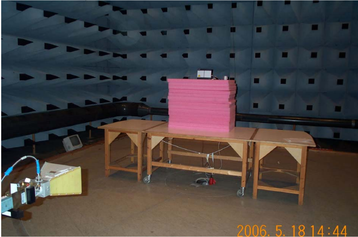
Photo A2.1 Equivalent isotropic radiated power (EIRP), Bluetooth module.
