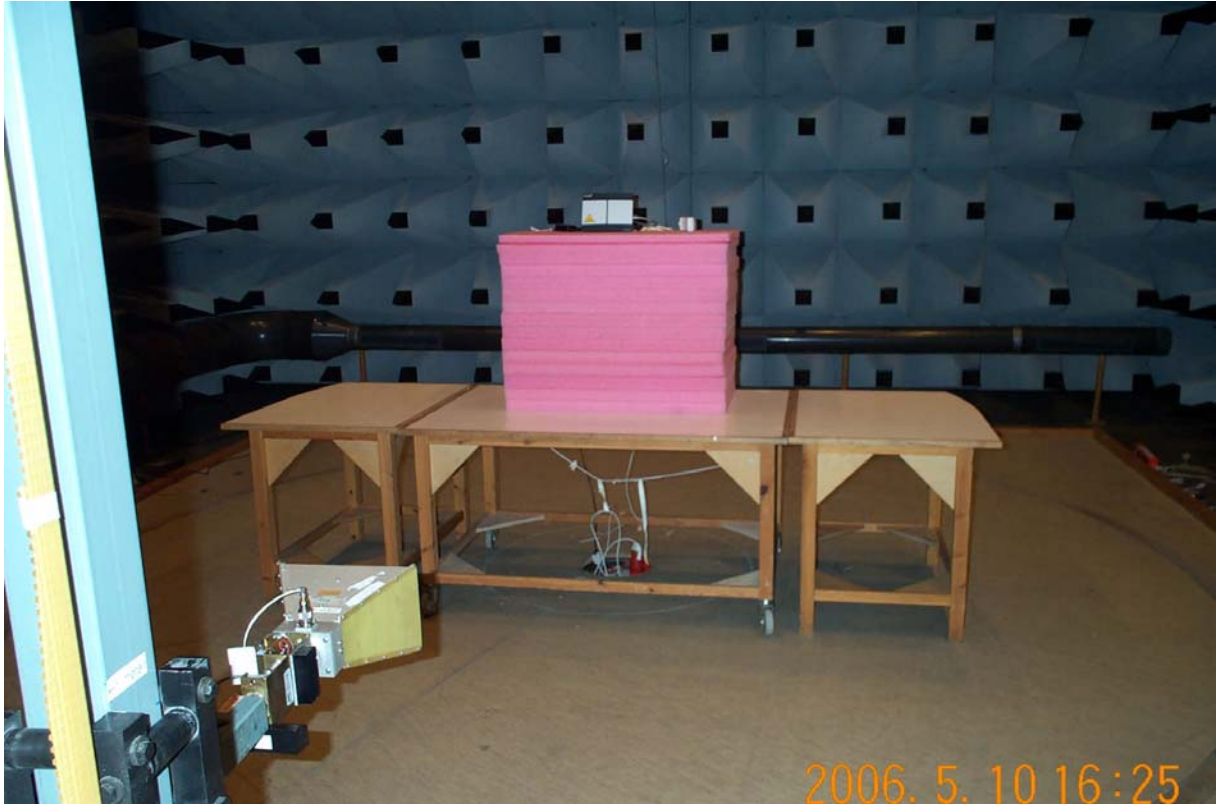
Photo A2.3 Transmitter spurious emission, Bluetooth module.
