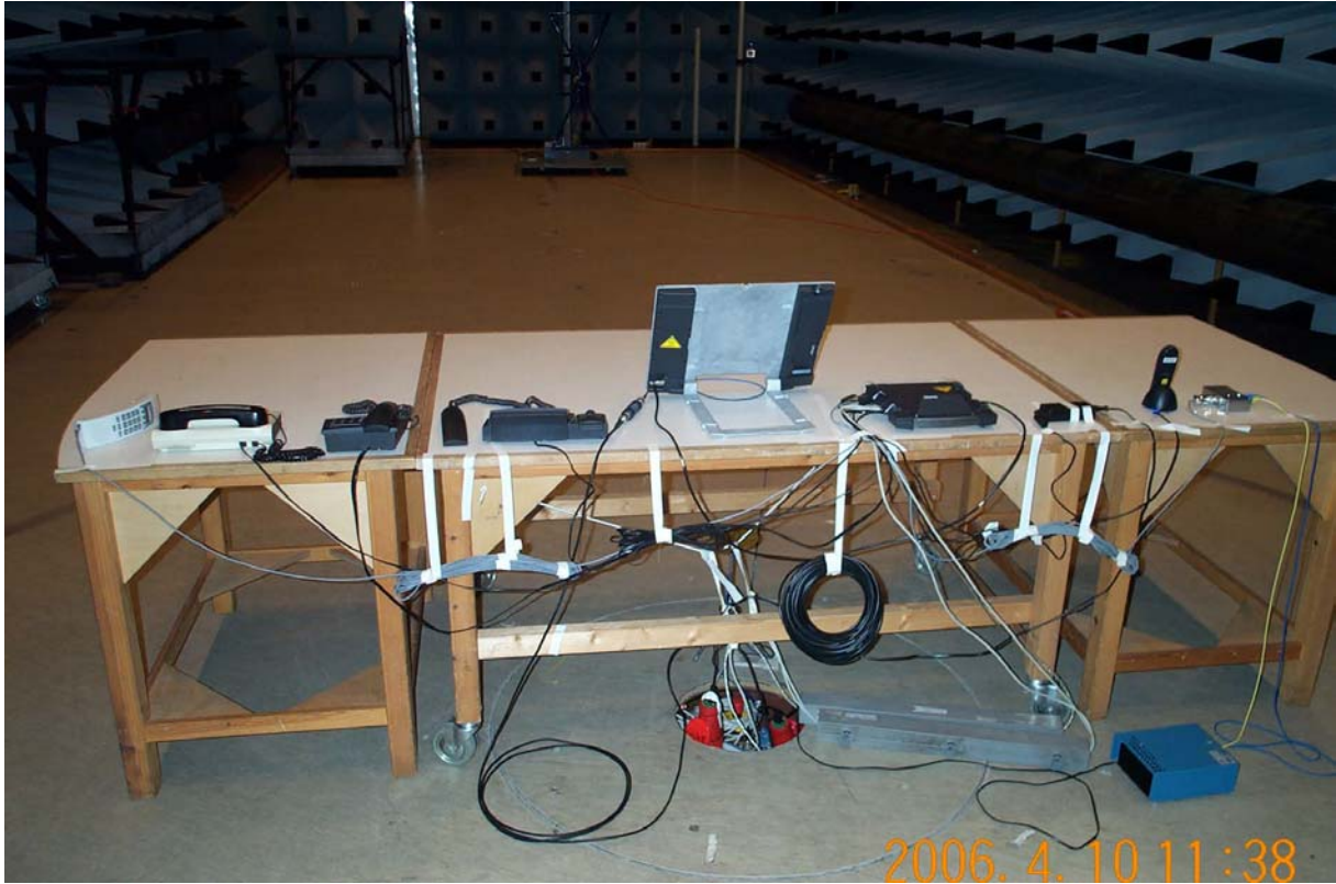
Photo A2.5 Unwanted emission measurements.
