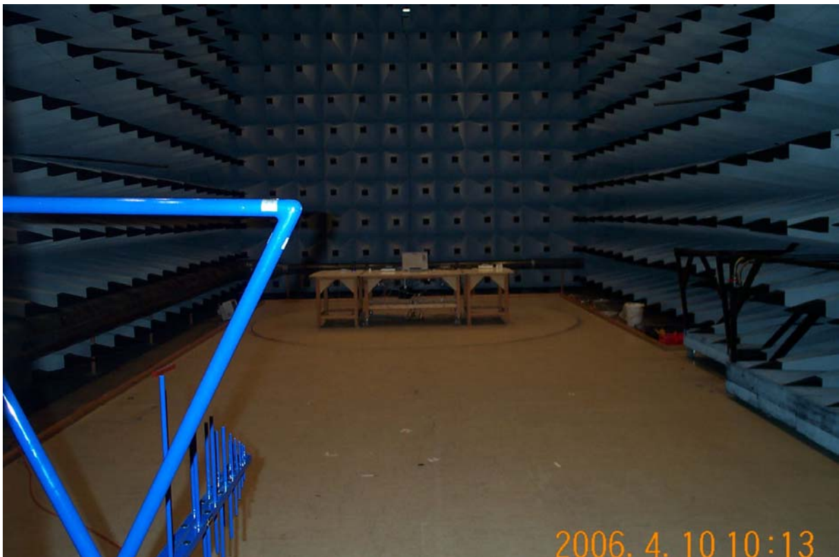
Photo A2.4 Unwanted emission measurements.
