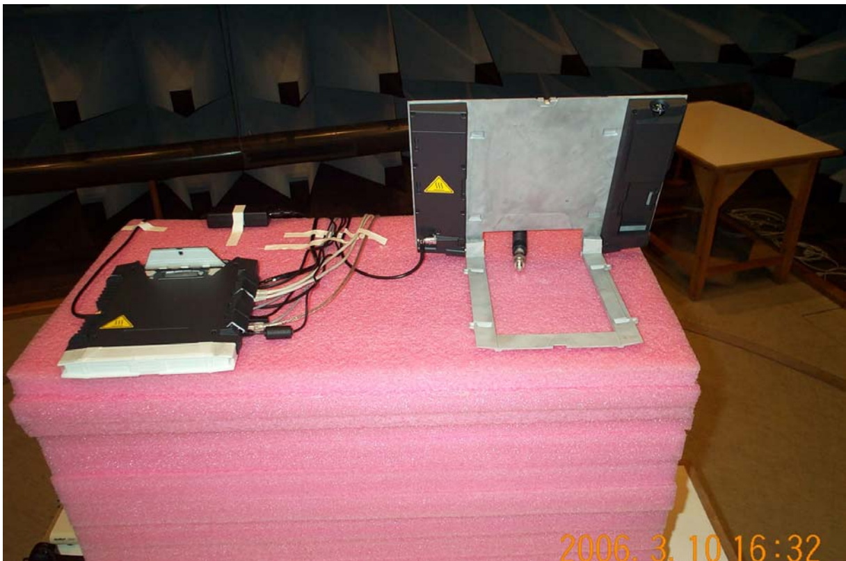
Photo A2.2 EIRP and transmitter spurious emission measurements.
